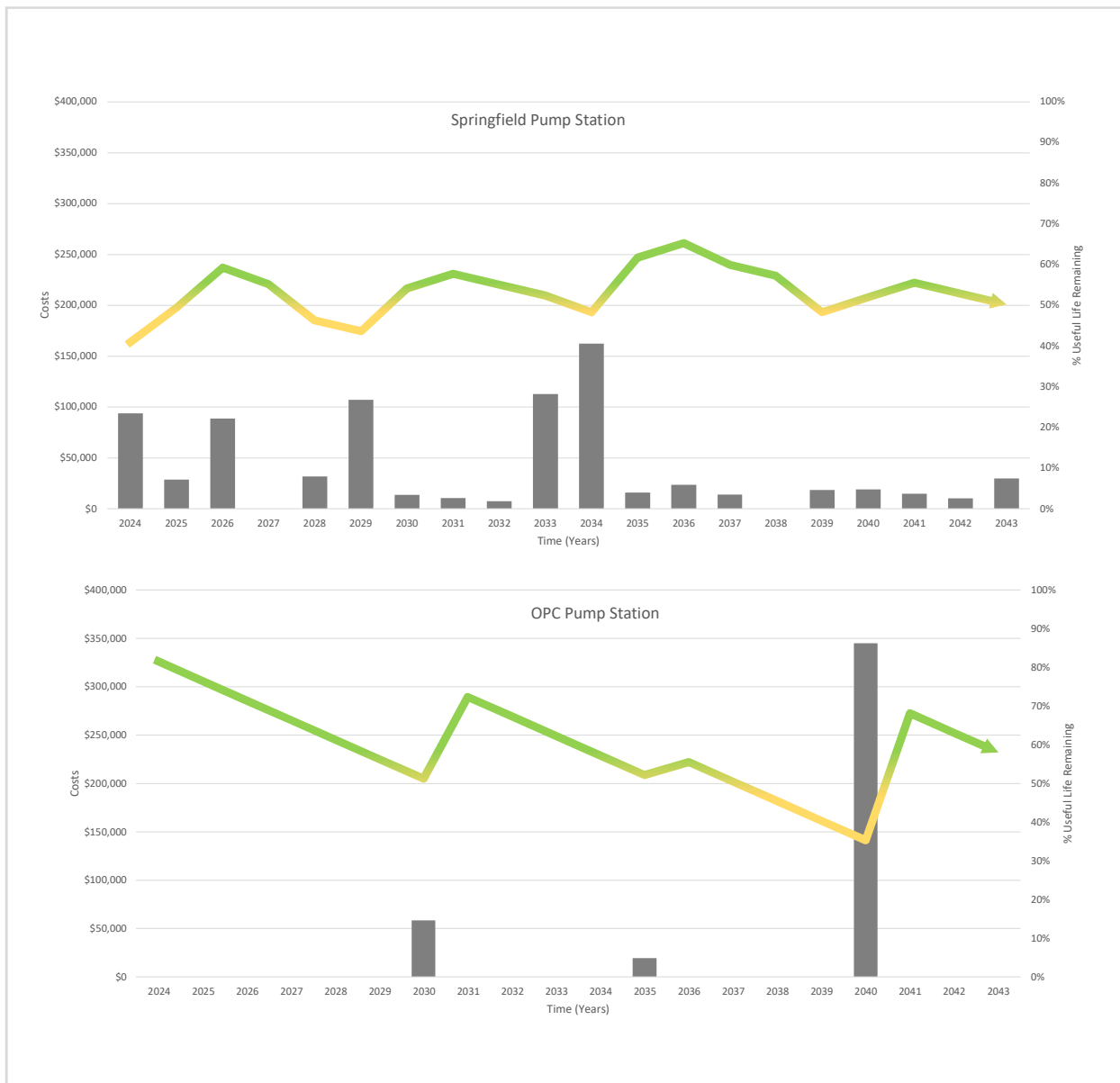
Figure 14 Condition Forecast – Pump Stations
